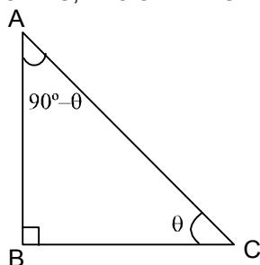
Clearly,  $\angle BAC$  and  $\angle ACB$  are complementary angles. We shall now express the trigonometric ratios of  $(90^\circ - \theta)$  in terms of those of  $\theta$ .
