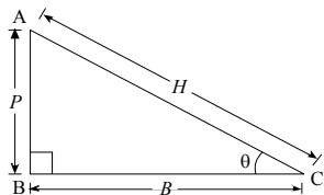
A right angled triangle is shown in **Figure**.  $\angle B$  is of  $90^\circ$ . Side opposite to  $\angle B$  is called **hypotenuse**. There are two other angles i.e.  $\angle A$  and  $\angle C$ . If we consider  $\angle C$  as  $\theta$ , then opposite side to this angle is called **perpendicular** and side adjacent to  $\theta$  is called **base**.
